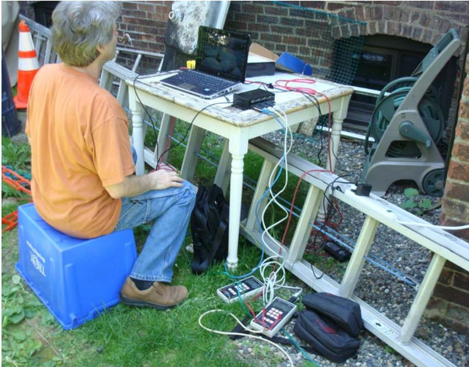
Test Setup for Side-by-Side Blower Door Test with Multiple Pressure and flow readings recorded simultaneously
