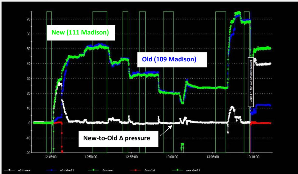
Figure 2. Pressure differences during fan test
