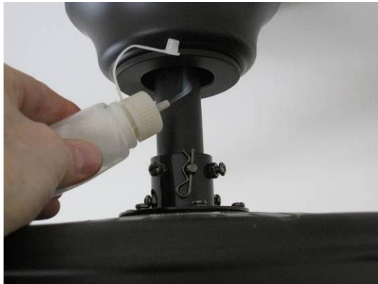
Air leak at ceiling fan
