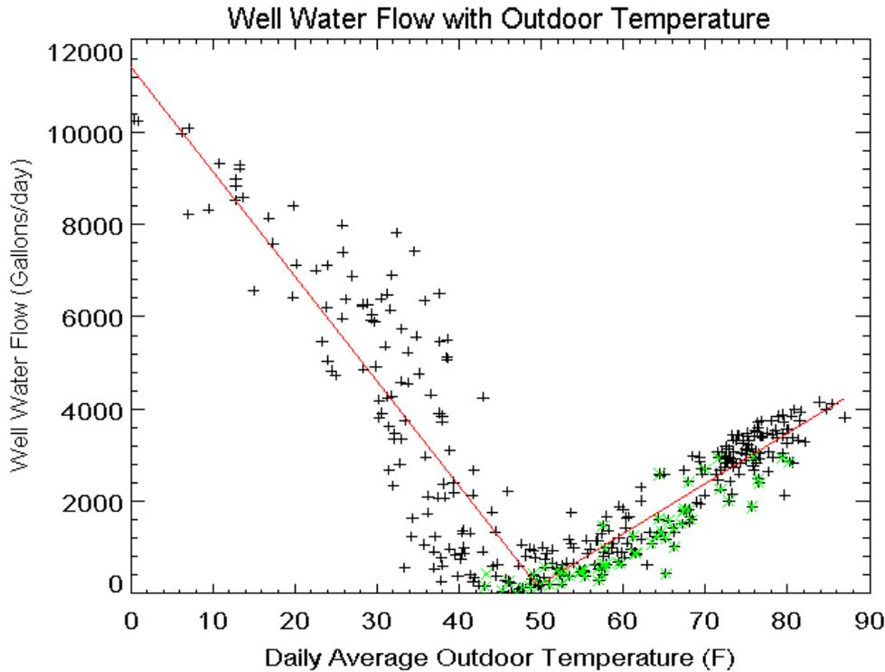
Figure 5. Well Water Use Relationship to Outdoor Temperature (Load)
