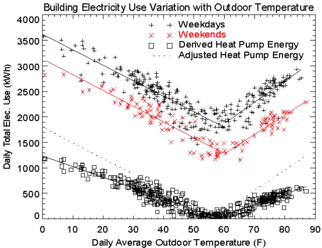
Figure 7. Total Building Electricity Use Relationship to Outdoor Temperature
