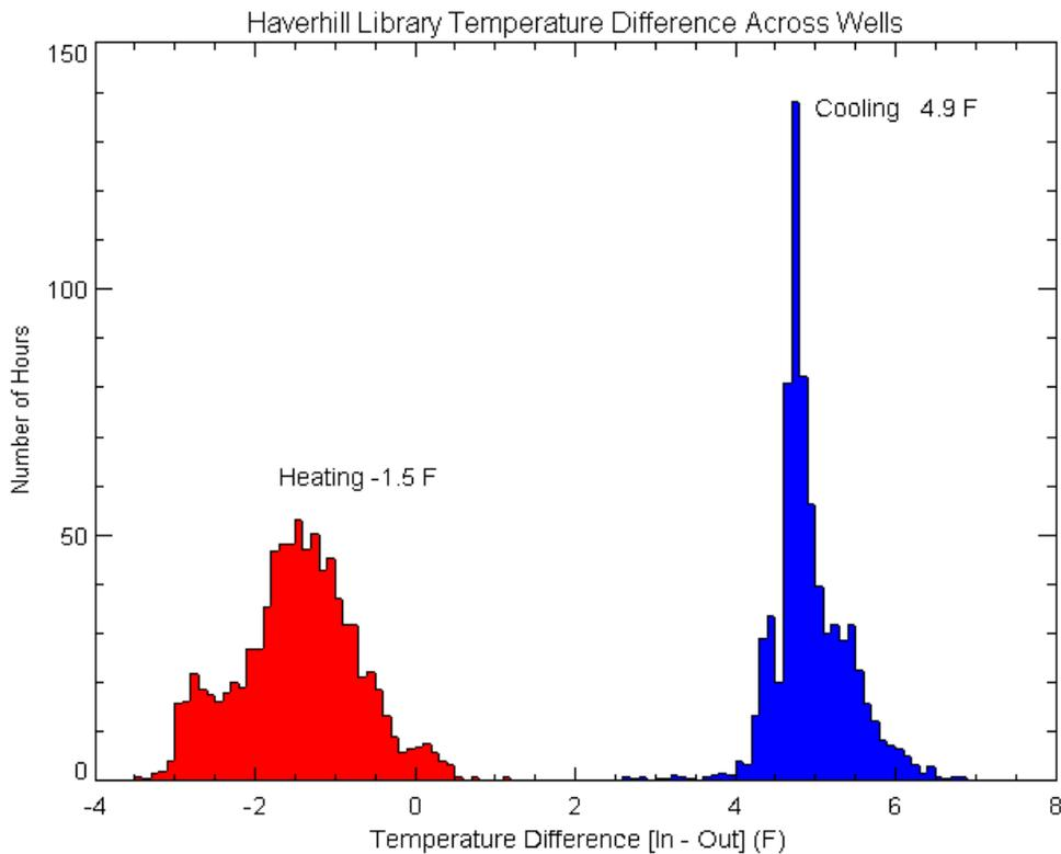
Figure 5. Temperature Difference Across Well Water Side of Heat Pumps
