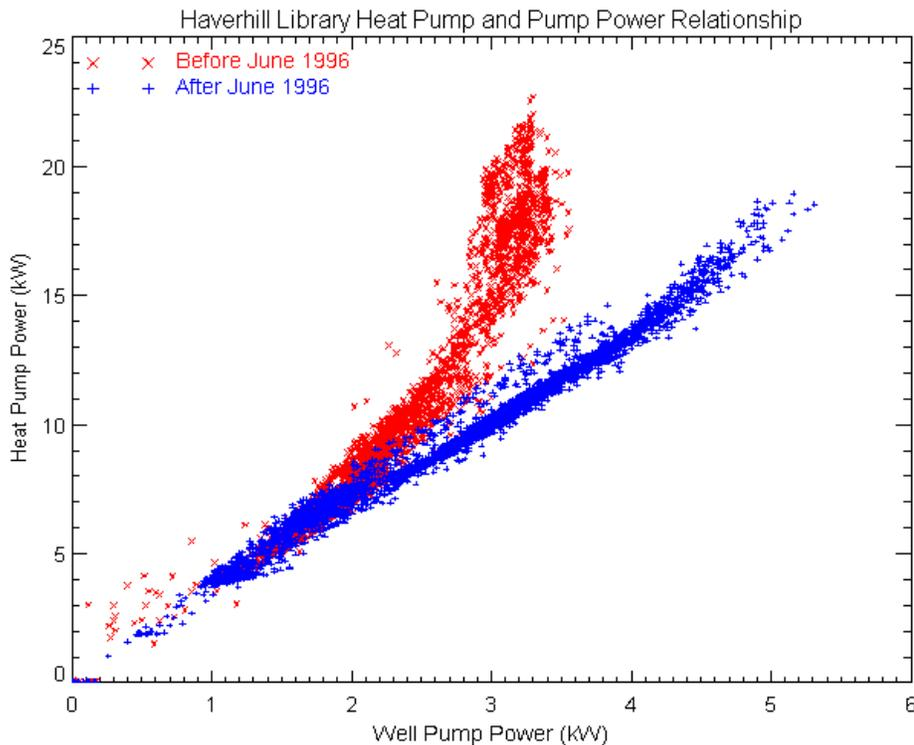
Figure 6. Heat Pump and Well Pump Power Relationship
