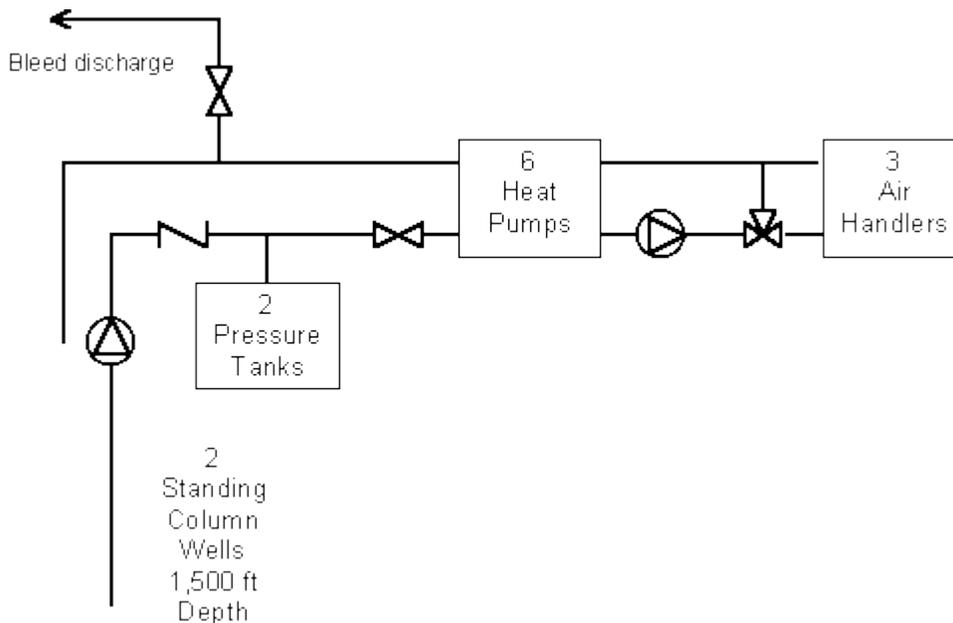
Figure 3. System Concept Schematic
