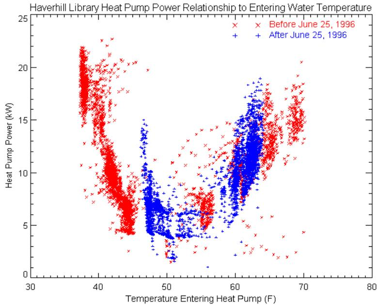
Figure 7. Heat Pump Power and Well Water Temperature Relationship
