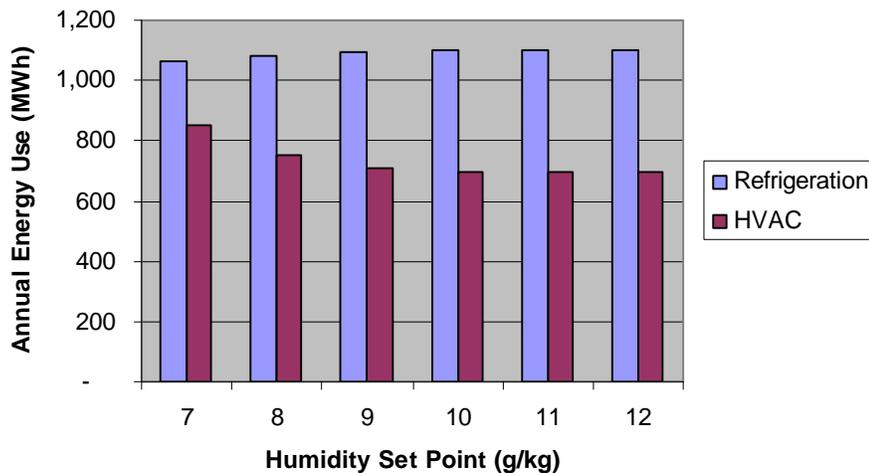
**Figure 10. Impact of Dehumidification Set Point on Refrigeration and HVAC Energy Use**
