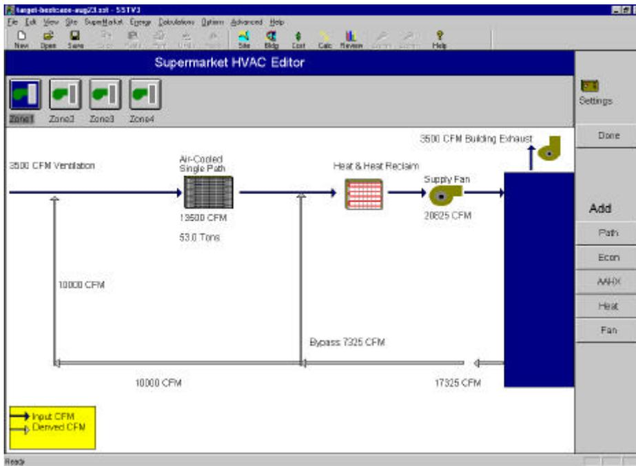
**Figure 3. HVAC System Editor with a Single Path System in Zone 1**
