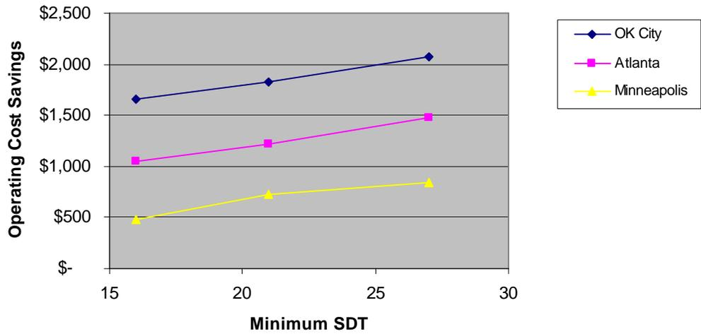
**Figure 9. Comparing Evaporative Condenser Savings in Various Climates**
