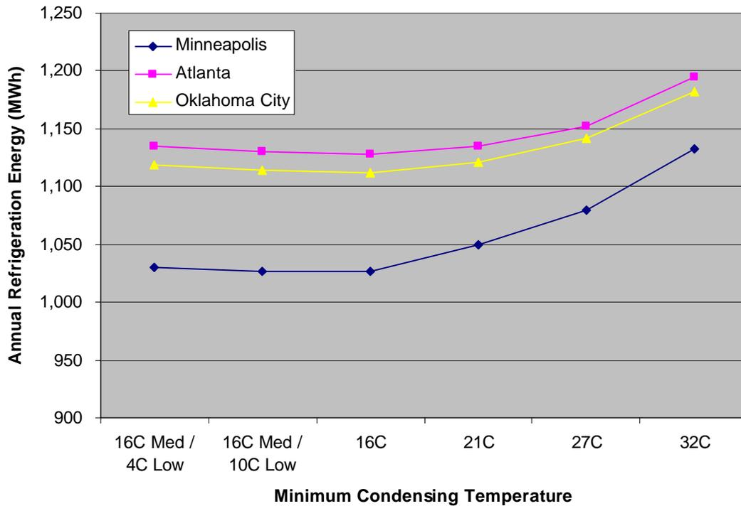
**Figure 7. Impact of Minimum Condensing Temperature on Annual Energy Use**
