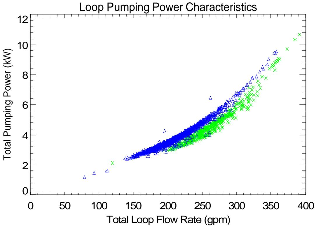
**Figure 14. Loop Pumping Power Verses Loop Flow Rates**
