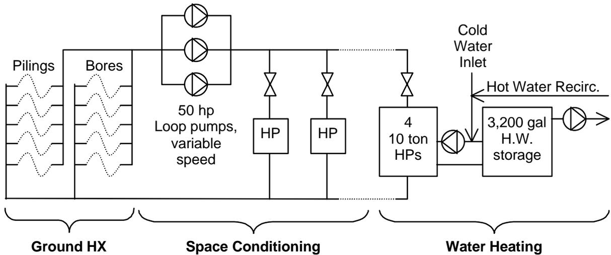
**Figure 3. Schematic Representation of Integrated Geothermal Space Conditioning and Water Heating System**
