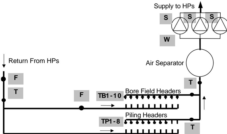
**Figure 7. Schematic Location of Monitored Data Points**
