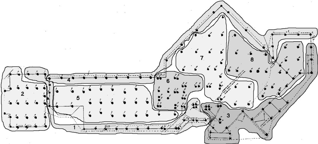
**Figure 2. Piling Location and Circuit Layout under Hotel**
