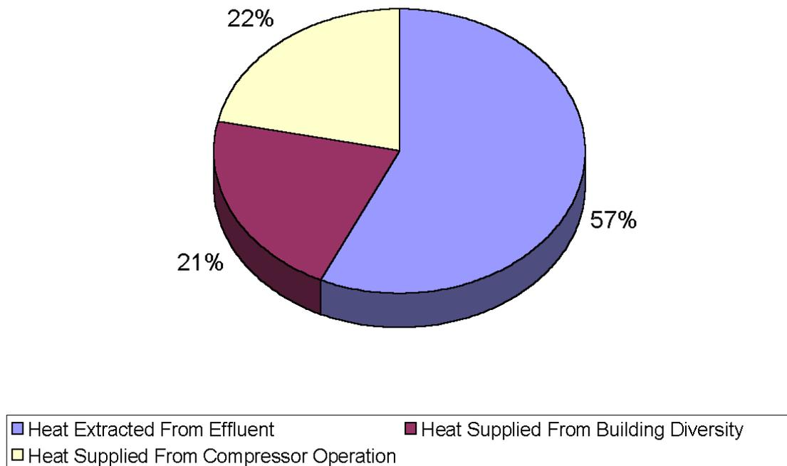
Figure 13. Heating Load Component Distribution
