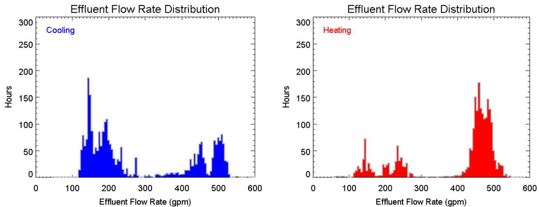
Effluent flow through the heat exchanger reached 709,000 gallons/day during the winter and 756,000 gallons/day during the summer. The total annual effluent flow was
