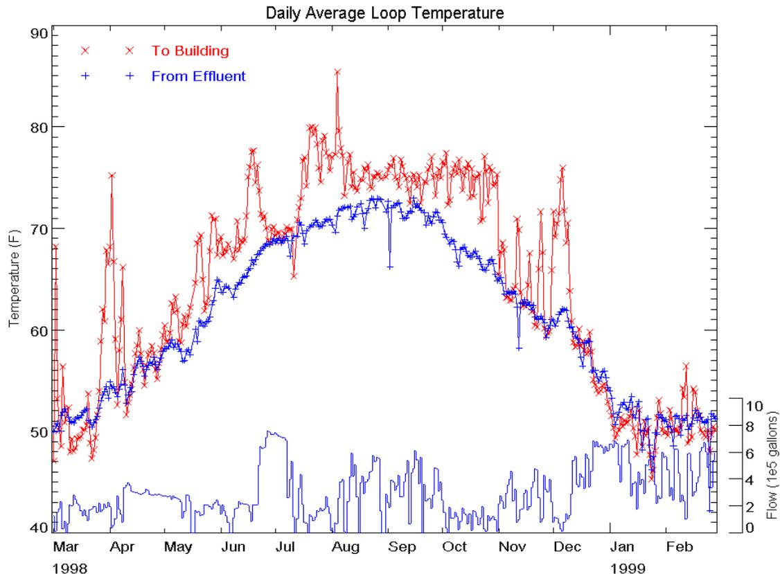
Figure 4. Daily Average Effluent and Building Loop Temperature
