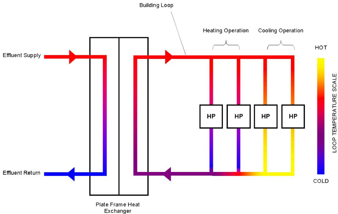
Figure 12. Schematic of Diversity Effect on Loop Temperature
