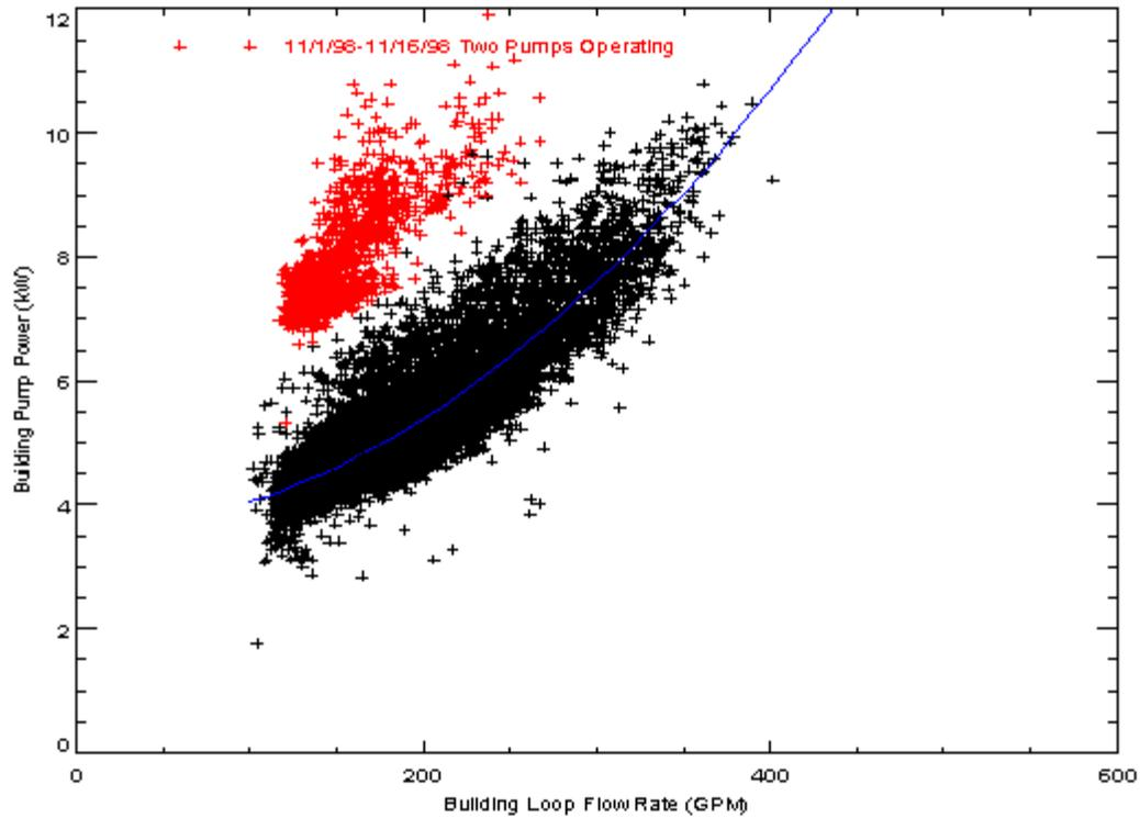
Figure 7. Building Pump Power Relation to Flow Rate
