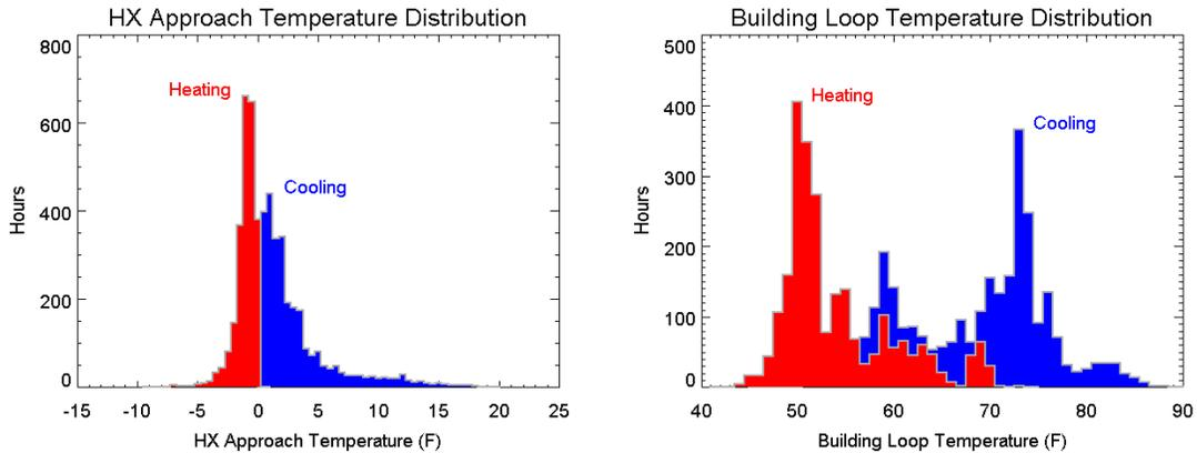
Figure 5. Building Loop Temperature Distributions
